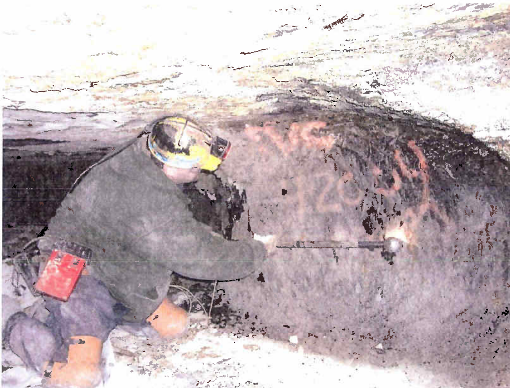
Figure 7: Striking rib with 10-pound sledgehammer to generate seismic source.
